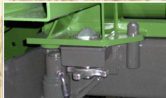
Twist-Lock locking system with parking stand holder.
