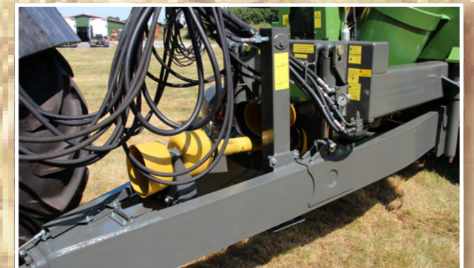
Hydraulic parking stand and hydraulic drawbar suspension.
