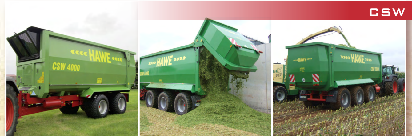
Cargo push-off trailer body with 40 or 50 cubic metres capacity.
