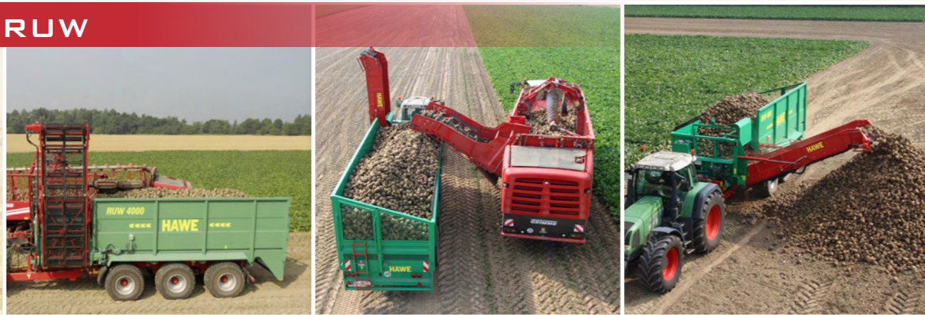
beet transfer trailers bodies with 28 (Tandem) and 40 or 50 cubic metres (Tridem).
