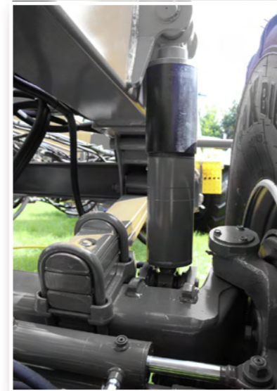
Running gear with hydraulic suspension available for all Tandem and Tridem chassis.
