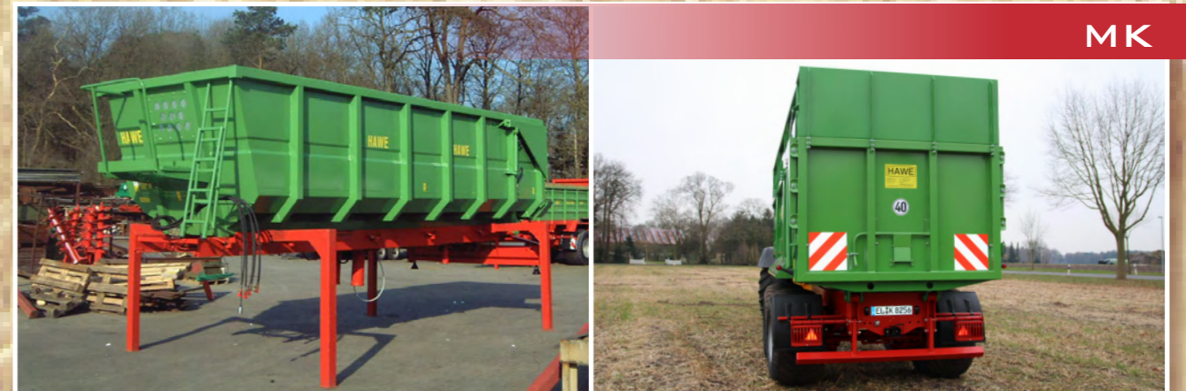
Dumper trailer bodies in different models from 22 to 44 cubic metres.
