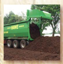
HAWE CSW 5000 with tridem running gear and parabolic suspension with self-steering for the first and third axle. Positive steering is available as an option.
