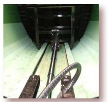
The bulkhead is operated by a multi-stage telescopic ram. The HAWE CSW experiences very little wear because moving parts are reduced to a minimum.
