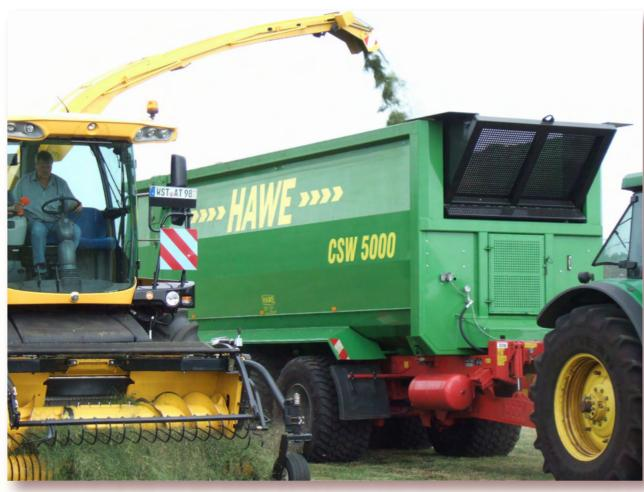
HAWE push-off trailers feature a strongly-built sheet steel body which is capable of withstanding high stresses. The bulkhead is operated by its own on-board hydraulics which are actuated by an electro-hydraulic remote control system. Two models are available with a capacity of 40 or 50 cubic metres.
