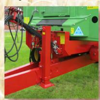
Hydraulic parking stand and hydraulic drawbar suspension.
