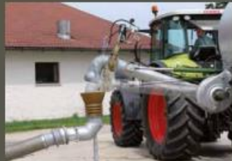
Suction nozzle (optionally with 8" turbo filler) Possible on left or right. With docking station; pressure sequence valve and hydraulic compressor changeover
