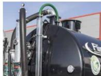
Internal pneumatic agitator, possible only in con-Plexigas fill level indicator rection with compressor. Slurry is homogenised
