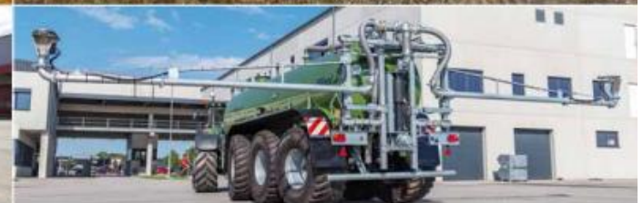
Nozzle boom spreader with maximum working width 21 - 30 m
