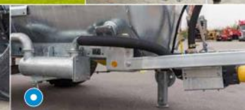
Silencer with oil separator
