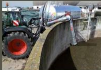
Elefant suction nozzle 8" Possible on left or right. Length 5000 mm with four-way control block. Turbo filler with telescopic extension 1500 optional
