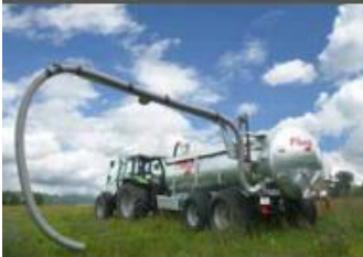
Lateral suction boom 4500mm length
