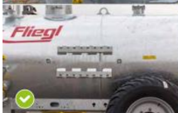
Mounting bracket for drag hose or drag shoe spreader STANDARD starting from 5000L
