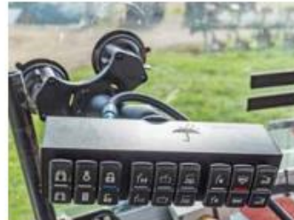
Control panel for Skate distributor and tank
