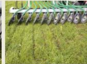
Jagged edge discs for better injection quality
