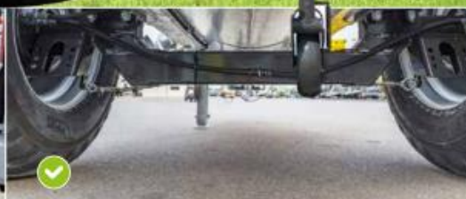
With offset axle starting from 5000 L: Low centre of gravity ensures optimal handling on slopes
