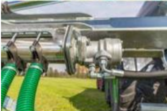
Oil motor for screw distributor with low wear and long service life. (Required oil quantity 20l max.)
