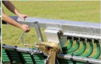
Storage box (with SKATE and GARANT) for foreign objects, emptied mechanically or hydraulically
