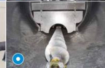
Hydraulic internal agitator with paddle screw for optimum homogenisation of the slurry (recommended for pig manure)
