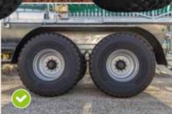
Wheel arch and tyres Tyres 750/60-R30.5* Optional: Rear tyres 750/60-R30.5* Front tyres 850/50-R30.5
