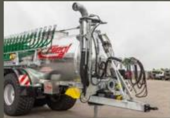
Pump tank suction nozzle 8"
